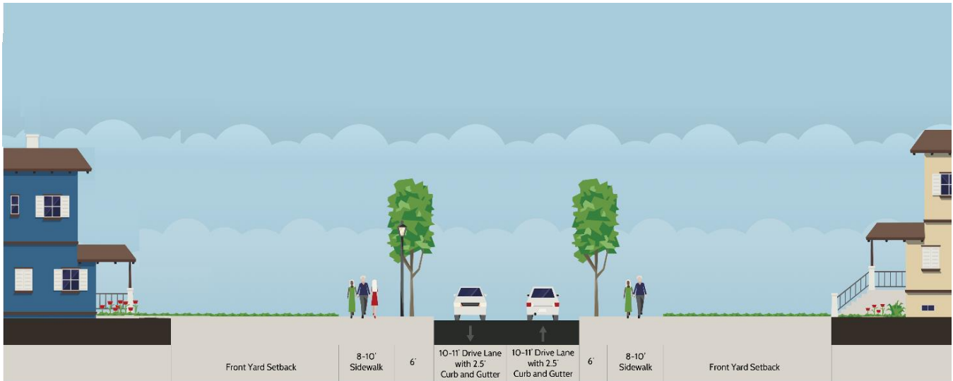
Figure 19 Proposed Typical Section for Local Street in School Study Area
