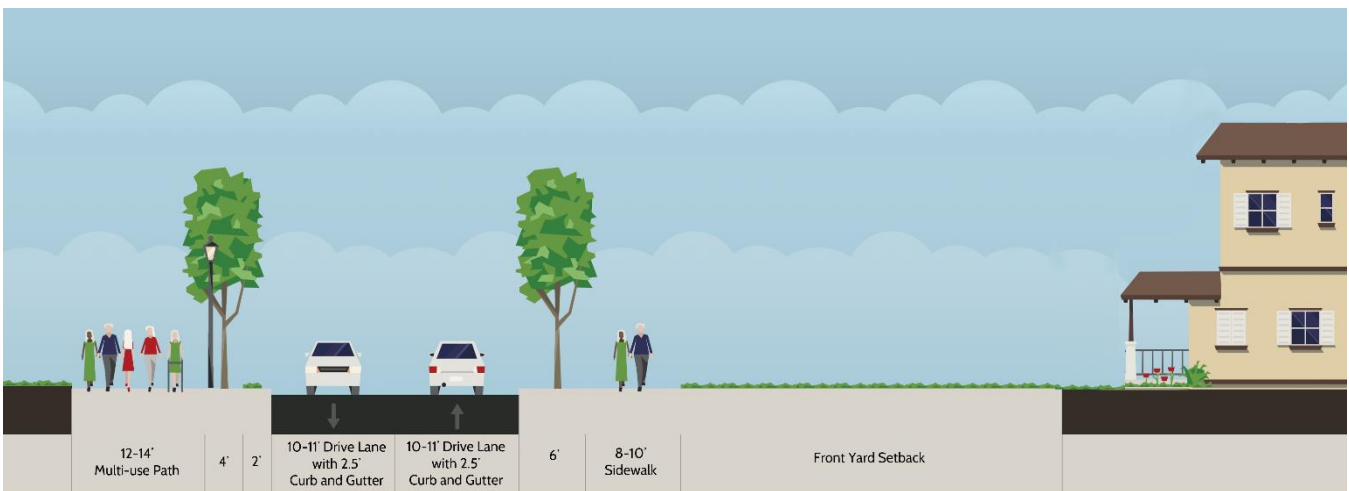
Figure 19 Proposed Typical Section for Local Street in School Study Area
