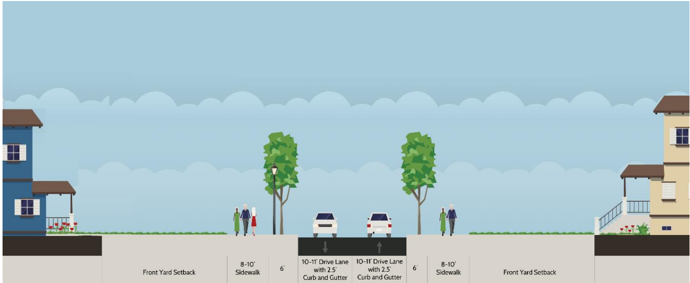
Figure 11 Proposed Typical Section for Local Neighborhood Street in Park Study Area
